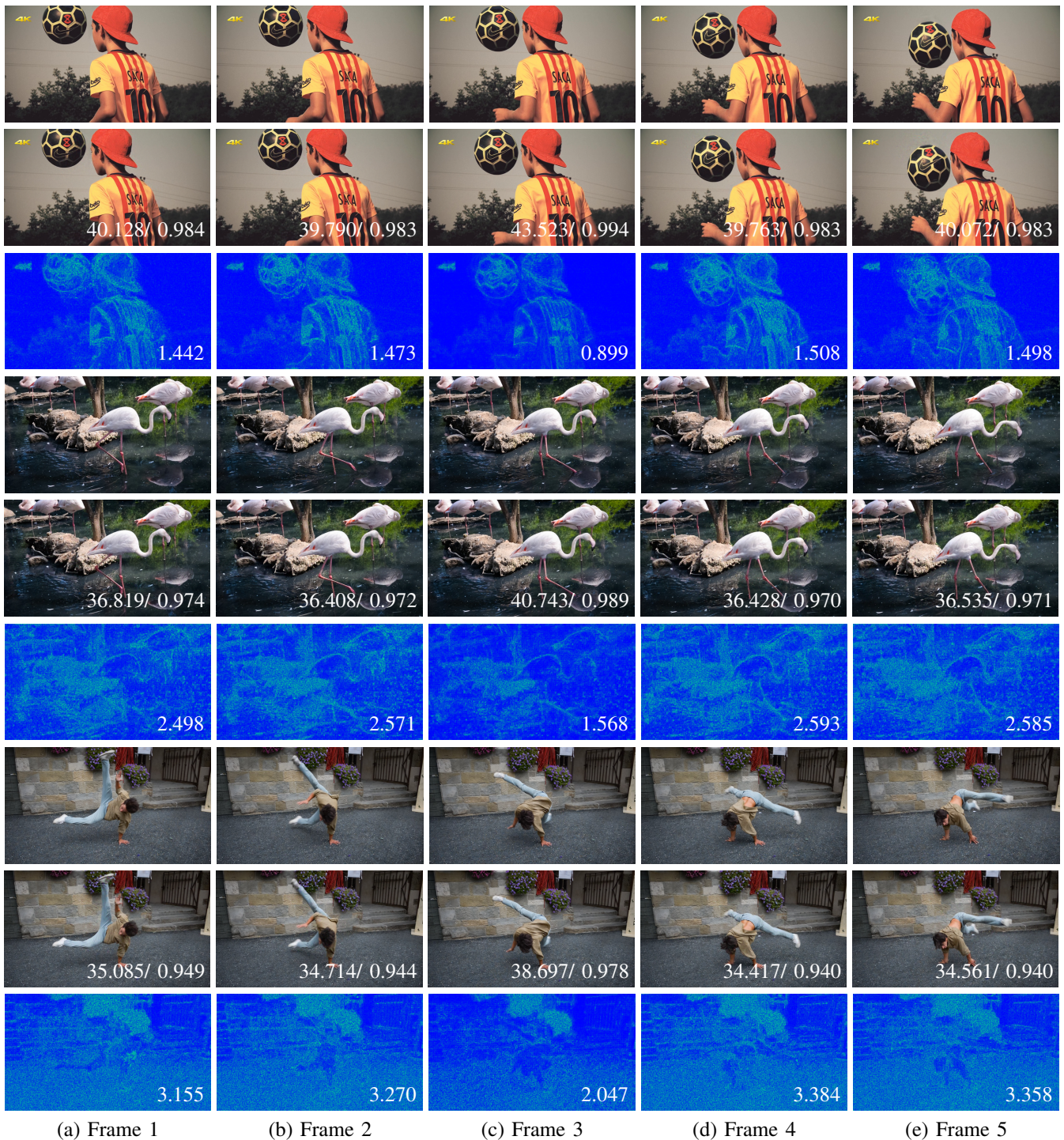
Fig. 13. Result gallery of the restored frames from the decoder. (a) to (e) contain of the complete input frames of the video. For each scene, images in the first row to the third row are the groundtruth frames, restored frames and the difference maps. PSNR, SSIM and MAE value are shown at the bottom right corner of corresponding images.
