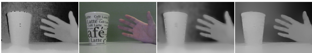
Figure 8. Depth map restoration with RGB image as guidance. Compared with [4], our method completely removes the background noise and does not blur edges.
