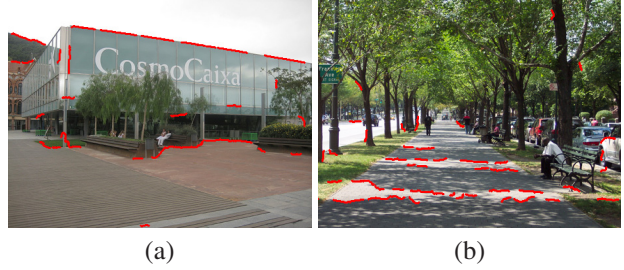
Figure 5. Shadow detection results of [8] for (a) a cloudy image and (b) a sunny image. Shadow detection in cloudy images is vulnerable to false detection.
