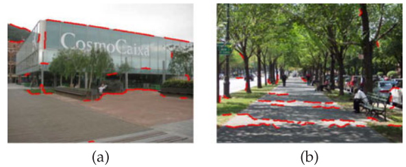
Fig. 5. Shadow detection results of [25] for (a) a cloudy image and (b) a sunny image. Shadow detection in cloudy images is vulnerable to false detection.
