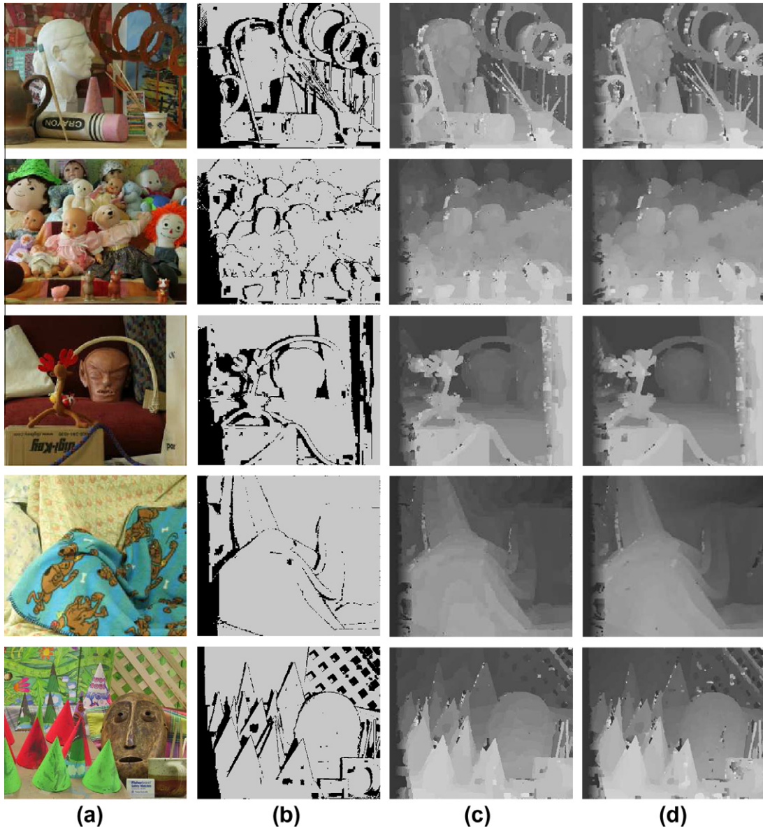
Fig. 10. Stereo matching examples. (a) Reference image in each image pair. (b) Occlusion map. (c) Disparity map obtained only using the low resolution images. (d) Disparity map estimated by our upsampling framework.
