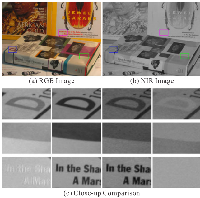
Fig. 1. Appearance comparison of RGB and NIR images. (a) RGB image. (b) Corresponding NIR image. (c) Close-ups. The four columns are for channels R, G, B, and NIR.
