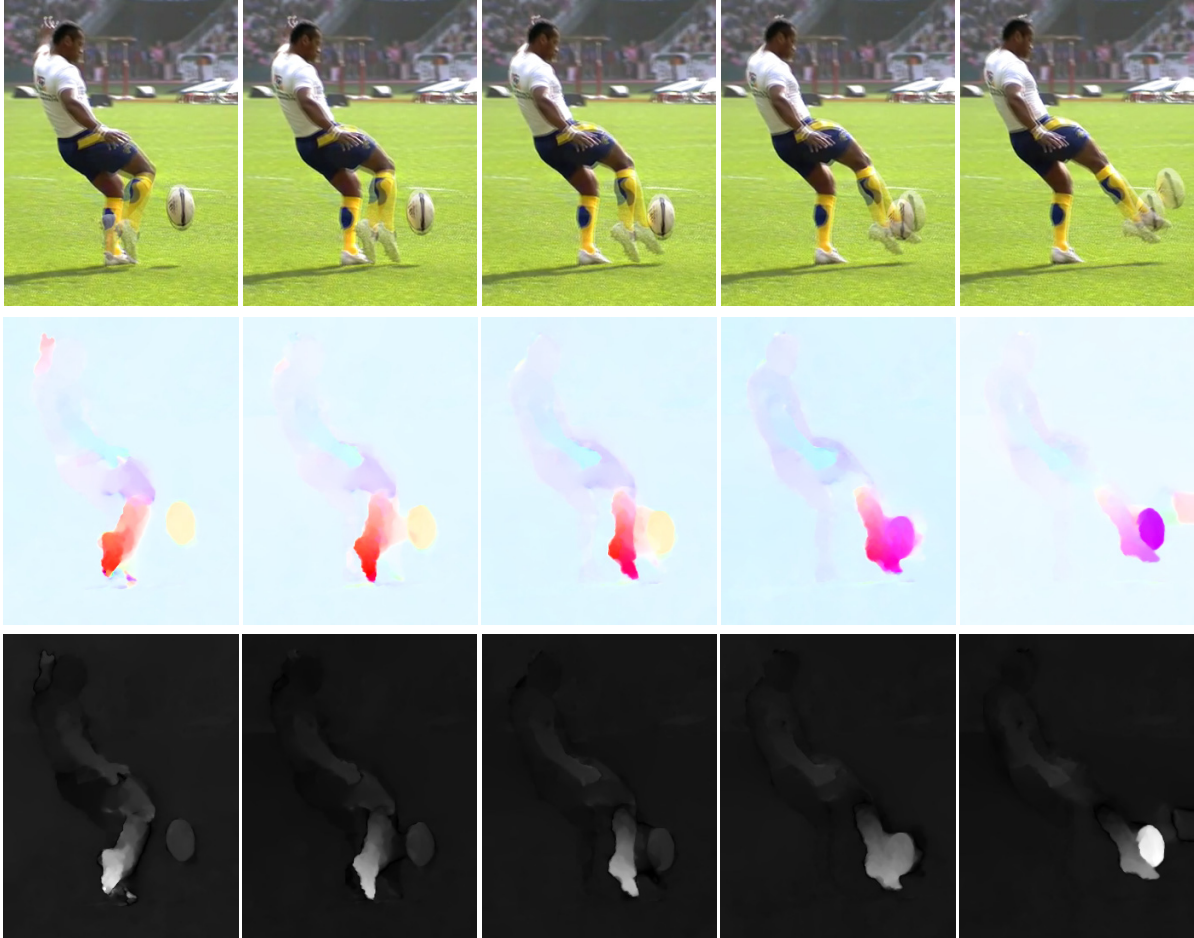
Fig. 16. Optical flow estimation in consecutive frames in a low-frame-rate sequence. First row: two-body-overlaid images to visualize the large displacement. Second row: our flow estimates. Third row: magnitude maps.
