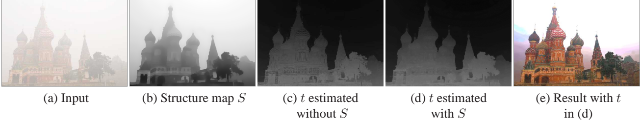
Figure 3. Structure layer extraction and its importance in transmission estimation compared to defining w_d on the input image I .
