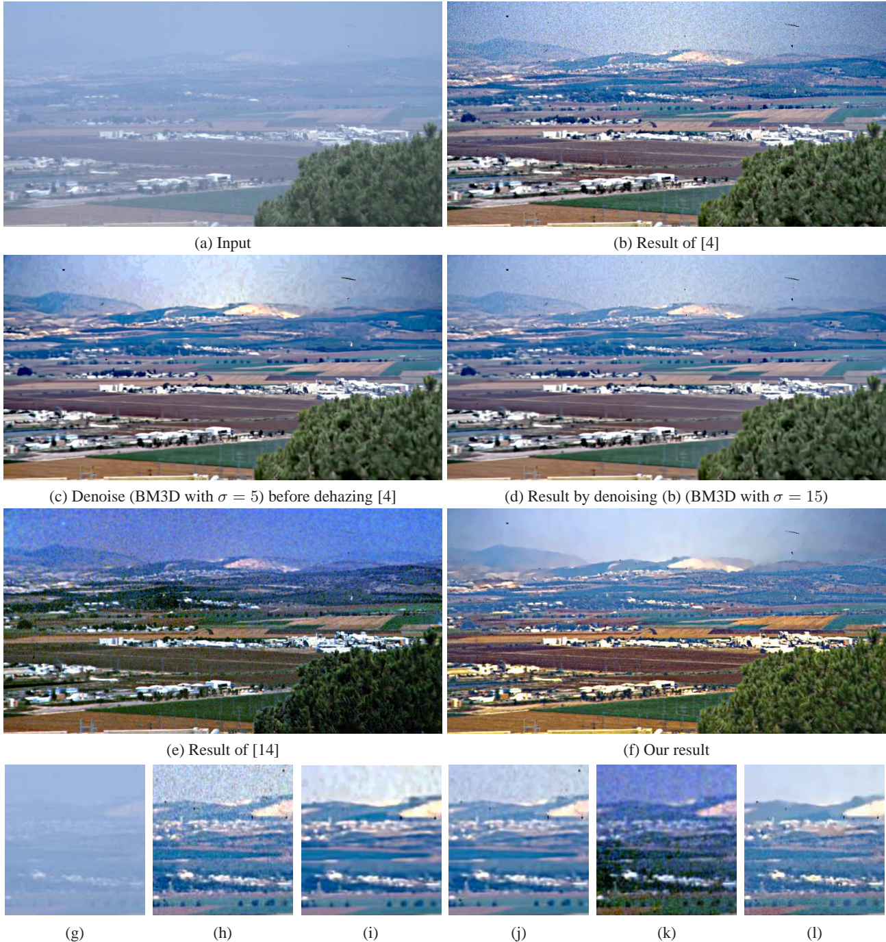
Figure 8. A dehazing example. Given input (a), our method produces the result (f). It not only removes intensive noise, also retains a great amount of details as well. Close-ups are shown in the last row.
