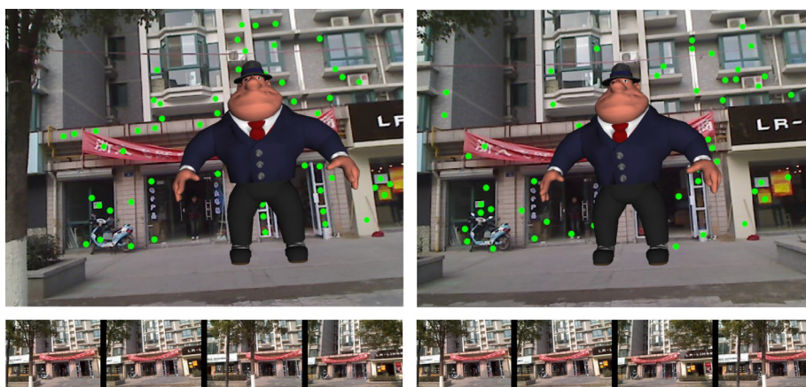
Fig. 9. The online camera tracking results of the “Street” example. Top: online images with the inserted virtual objects. Bottom: the computed candidate keyframes.
