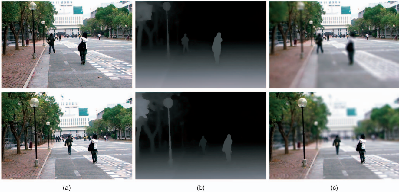
Fig. 12. Depth-of-field. (a) Two frames from an input video. (b) The recovered depth maps. (c) The result of changing the depth-of-field.
