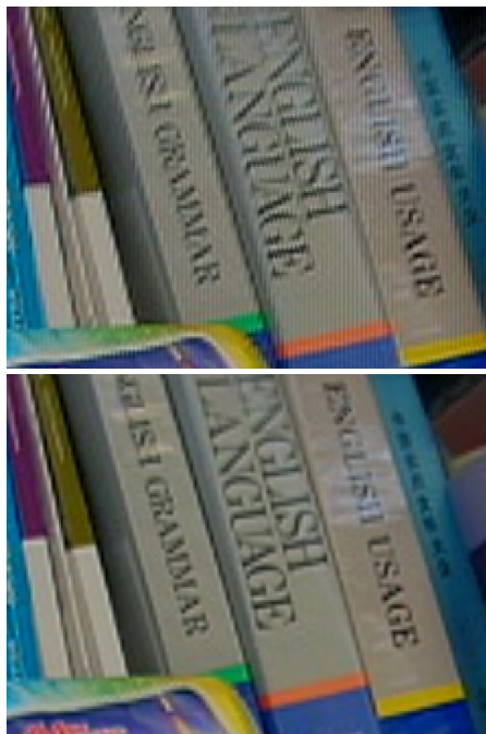
Fig. 4. A comparison of the resulting super-resolved images. The enlarged region located near the middle top of the left view is shown. The upper and the lower picture are the results by Irani's algorithm and our approach, respectively.
