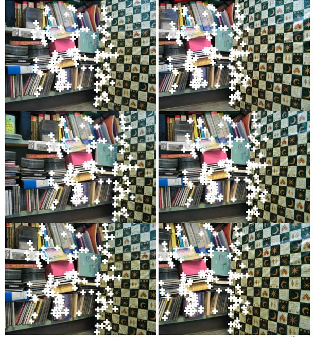
Fig. 8. The top row: A map of the point features extracted from the 1<sup>st</sup> image pair of the stereo image sequence. The middle row: The re-projections of the extracted point features in the 35<sup>th</sup> image pair. The bottom row: The re-projections of the point features in the 100<sup>th</sup> image pair. Note that the left and the right column show the images captured by the left and right camera in the stereo system, respectively.
