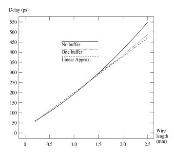
Figure 1: A simple experiment to illustrate the relationship between wire delay and wire length.
