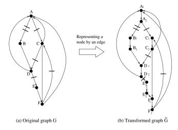
Figure 4: Representation of gates by wires.
