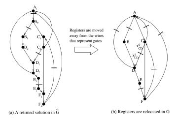
Figure 5: Relocation of registers retimed into a gate.
