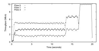
Figure 12: Providing differential bandwidth allocation using XCP. Three XCP flows each transferring a 10 Mbytes file over a shared 10 Mb/s bottleneck. Flow 1' s price is 5, Flow 2' s price is 10, and Flow 3' s price is 15. Throughput is averaged over 200 ms (5 RTTs).
